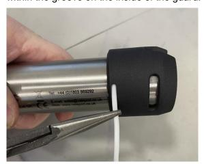
It is very tight and difficult to get all the way around the Hyperion housing. A spot of silicone grease will help.
