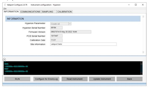
Press the Read Instrument button to interrogate the instrument to upload all the current settings.
