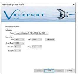
This setting has no effect on Hyperion Fluorometers with MK2 PCBs. All Hyperions supplied after November 2020 (Serial No: 75100) have MK2 PCBs. If you get an error concerning #400 commands change the instrument to: **Hyperion X - .SN > 75100 Nov 2020** in the drop down menu.
