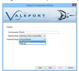
For dye tracing applications, we recommend using the Hyperion at the default range, that is, high gain/sensitivity to reduce the quantity of dye required and, therefore, the visibility / load on the environment and or disposal costs.
