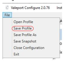
A new feature for ver 2.0.76 is the Snapshot. This, unlike the Profile is a text file that includes all details about the instrument including those that are not an instrument setting such as serial numbers, calibration dates and site information
