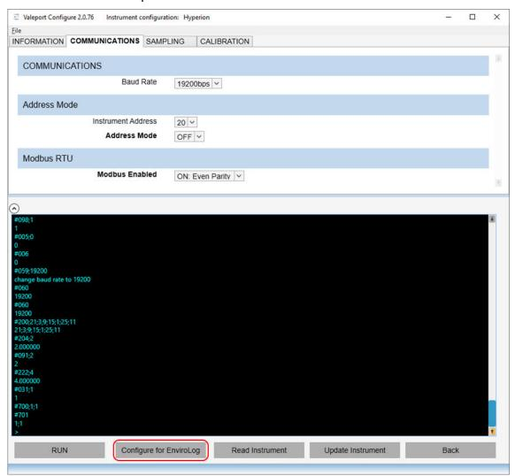
Once complete the Hyperion is setup and ready to be interfaced to the EnviroLog system. You must ensure that if you are using multiple instruments each has a different Address.
