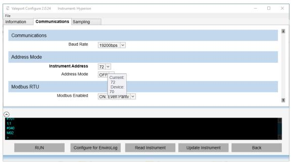
Once you have made all your changes press Update Instrument to upload the new configuration into the instrument
