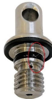
Excessive grease has been applied to the O ring and as a result, debris has become associated with it. Debris of this kind can provide a channel for water to seep through into the SWiFT
