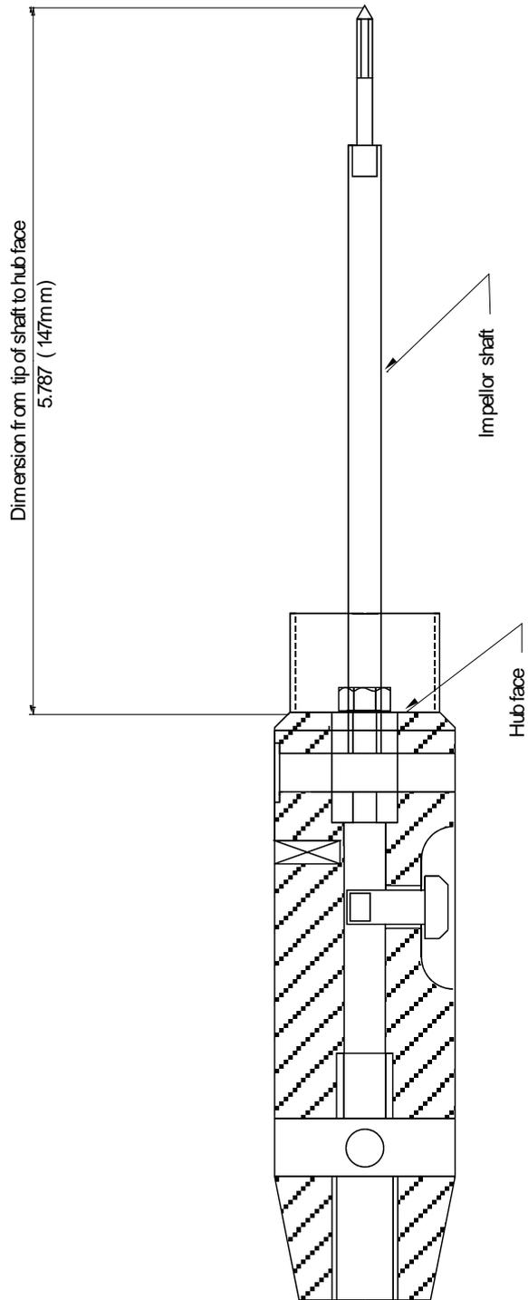
Figure 2 – BFM001 impeller shaft setting
