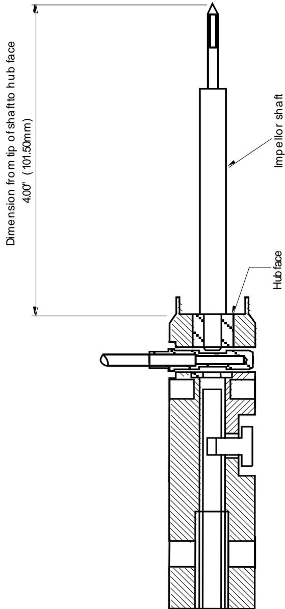
Figure 4 – BFM002 impeller shaft setting
