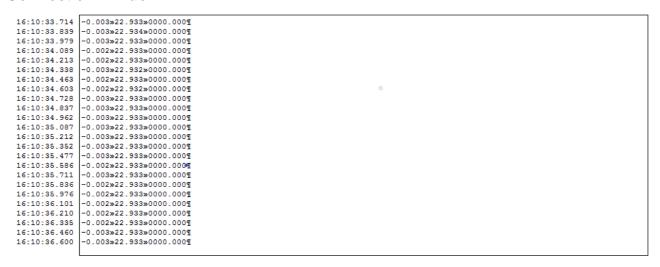
The connection window shows any communications between the PC and the connected instrument. In the example above the time stamping is enabled. Once the window is full, it will scroll with any received data. Data can be highlighted, selected, copied and pasted.
