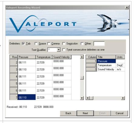
For data recorded on instruments without a Real Time Clock, there is the option to append a timestamp to each record.
